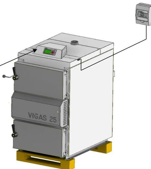
We insert the AK BUS E cable through the hole on the side of the top cover of the boiler and then insert it into the free socket on the AK4000 power board. For **DPA** boilers, it is necessary to use the socket on the pellet expander module **AK4000EP**, which is located under the pellet hopper (fig. 29).
